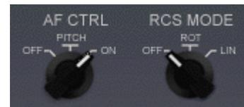
The RCS MODE selector sets the Reaction Control System mode which is used to control attitude in free space. During atmospheric flight, when aerodynamic control surfaces are active, the RCS is usually disabled. The selector can be set to OFF (RCS disabled), ROT (RCS in rotational mode), and LIN (RCS in linear mode).
