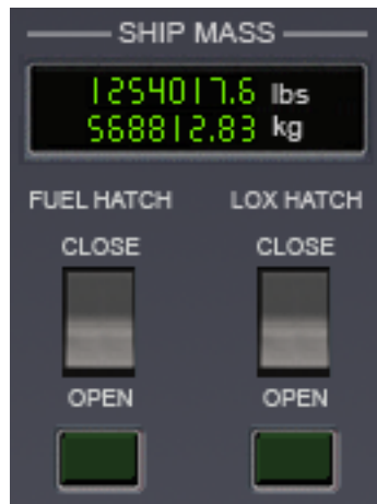
Ship Mass Display and Resupply Hatch Switches
